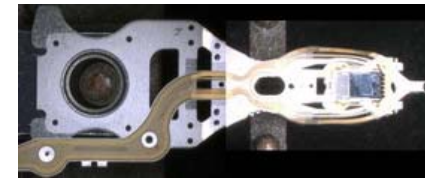
PZT's in Gimbal Area (shown photo above: CAT)
